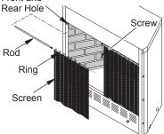
Figure 16 - Installing Fireplace Screen (Shown Without Fireplace Hood for Clarity)
